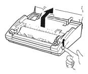
■ While pushing outward on each white tab, lift the Roller and out of the machine.
